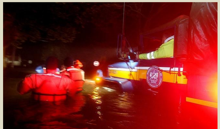
One of two converted surplus military cargo trucks used for high-water responses
